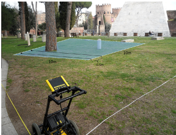
Fig. 3. The GPR surveyed area around the 'PO' column and the line spacing parameters. Note the presence of a pine tree inside the area.
